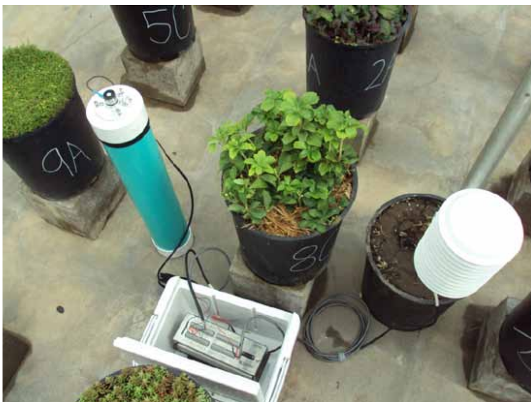
Figure 2. Environmental conditions (temperature, relative humidity, and photosynthetically active radiation) in the greenhouse were monitored.
