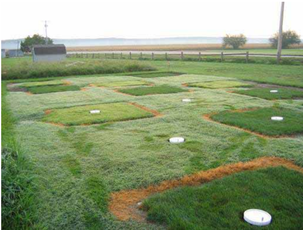
Figure 1. Plots of perennial ryegrass, zoysiagrass, and Bermudagrass. Measurements of N 2 O were collected from each plot with static surface chambers as shown.
