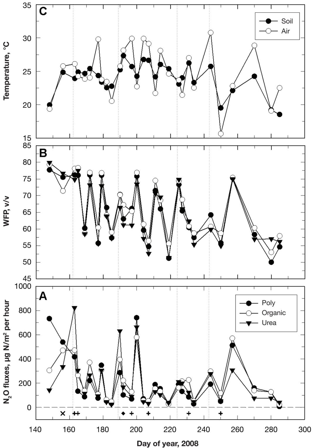
Figure 2. (A) Fluxes of  $N_2O$ -N from plots fertilized with polymer-coated urea (poly), organic nitrogen, and urea; (B) water-filled porosity (WFP) in the 0- to 6-in. profile; (C) average soil temperature at 2 in. among treatments and air temperature at 6.5 ft at sampling.
