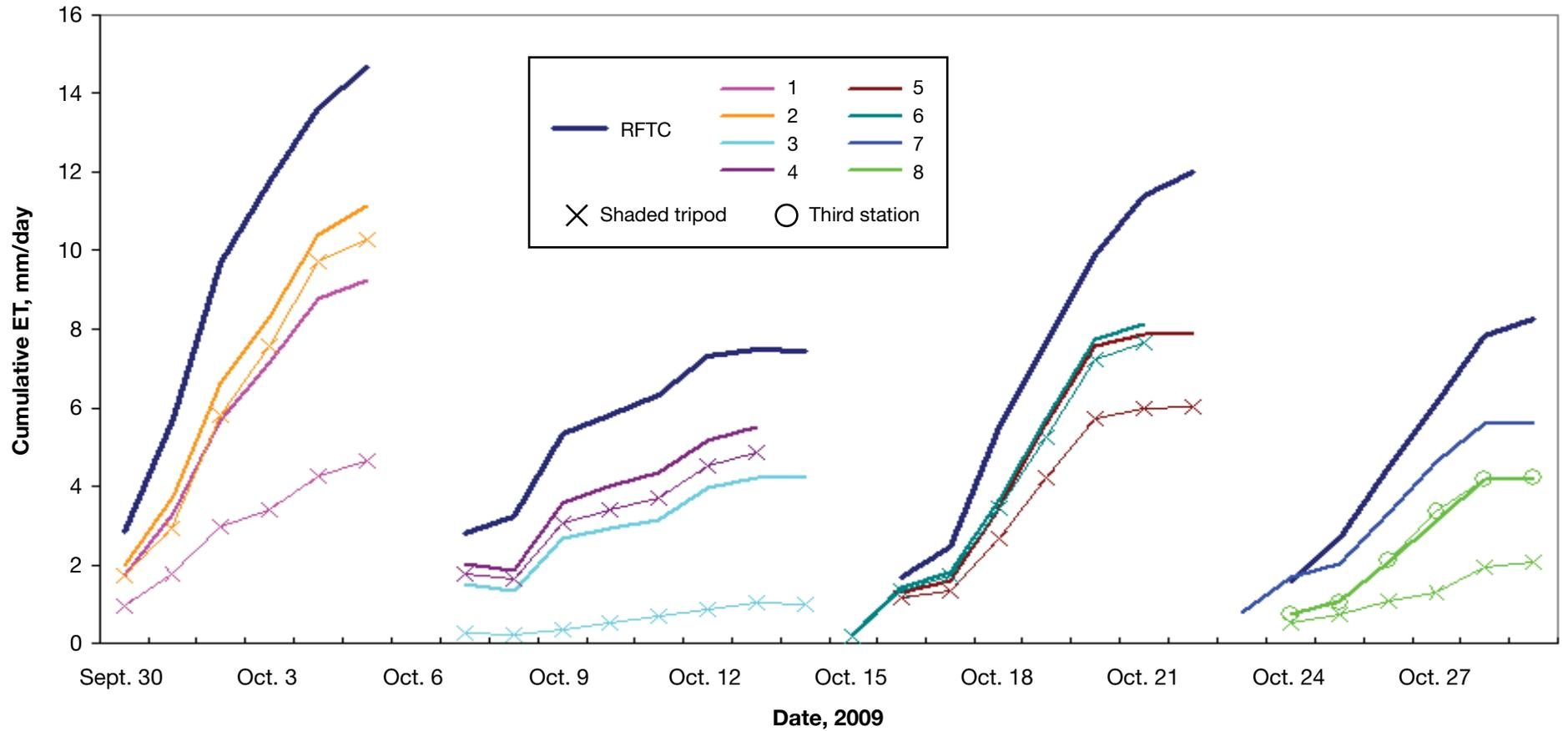
**Figure 5. Cumulative reference crop evapotranspiration (ET<sub>c</sub>) from all lawn-deployed tripods compared with that from the tripod at the Rocky Ford Turfgrass Research Center.**
