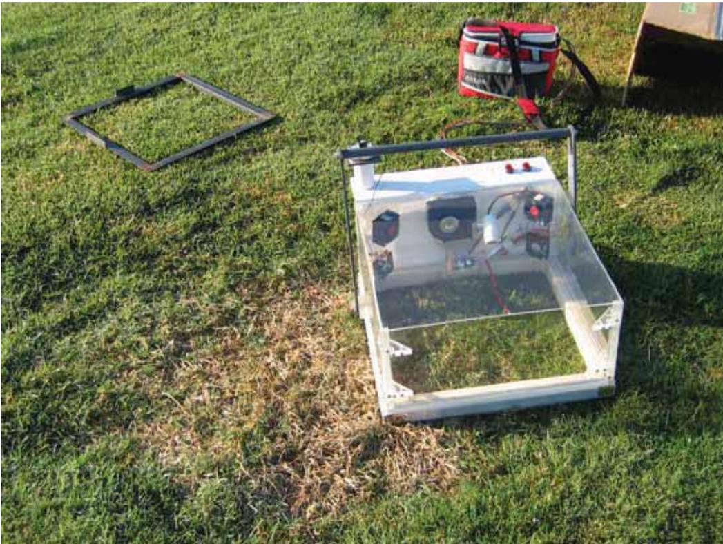
**Figure 1. Large chamber fabricated to measure CO<sub>2</sub> fluxes in turfgrass.**
