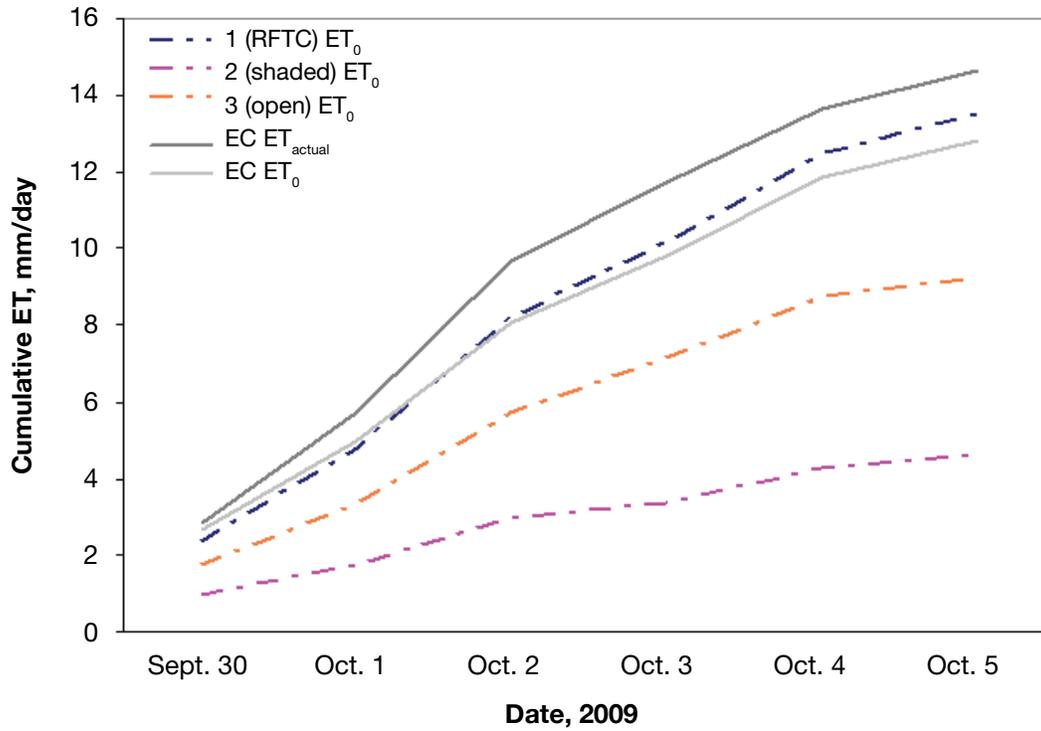
**Figure 4. Cumulative reference crop evapotranspiration ( $ET_0$ ) reported by three tripods during deployment on one property and cumulative  $ET_0$  and actual evapotranspiration ( $ET_{actual}$ ) as measured at the eddy covariance (EC) site.**
