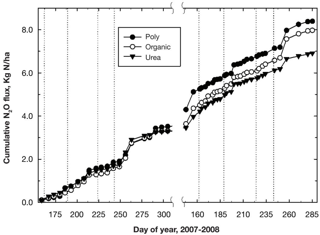
**Figure 3. Cumulative fluxes of N<sub>2</sub>O-N from plots fertilized with polymer-coated urea (poly), organic nitrogen, and urea.**
