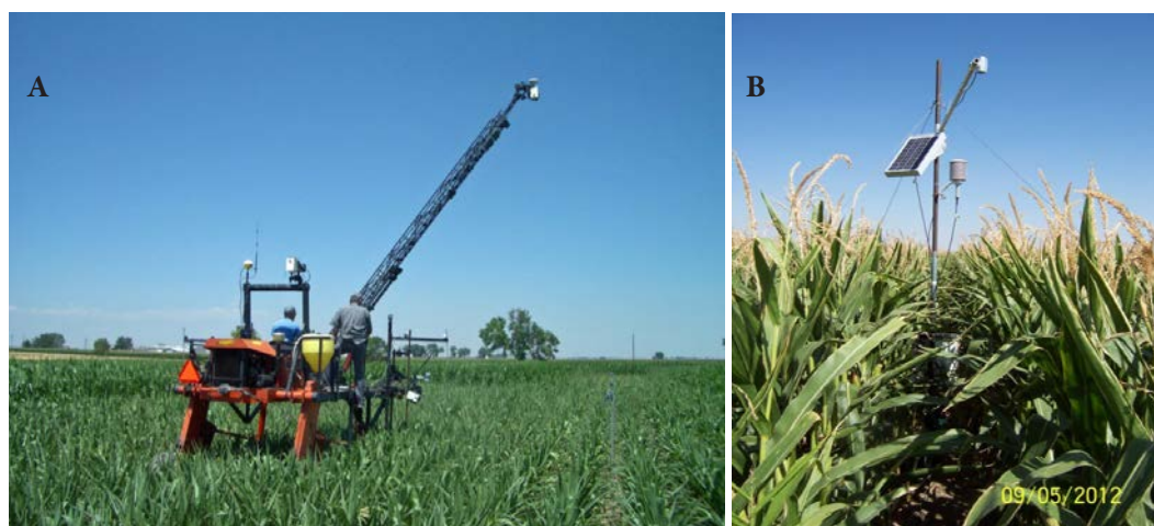
Figure 1. Ground-based remote sensing of canopy temperature using a thermal camera on a tractor crane (A), and ground-based remote sensing of corn canopy temperature using thermal infrared radiometers (B) at USDA ARS, Fort Collins, CO.
